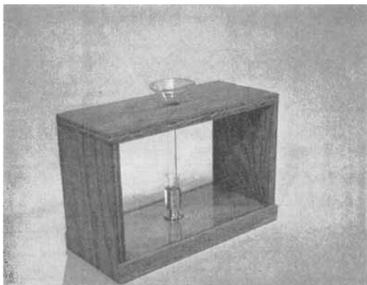
Fig. 1—Device to transfer cellulose from chromatoplates to capsules for oxygen ignition.
